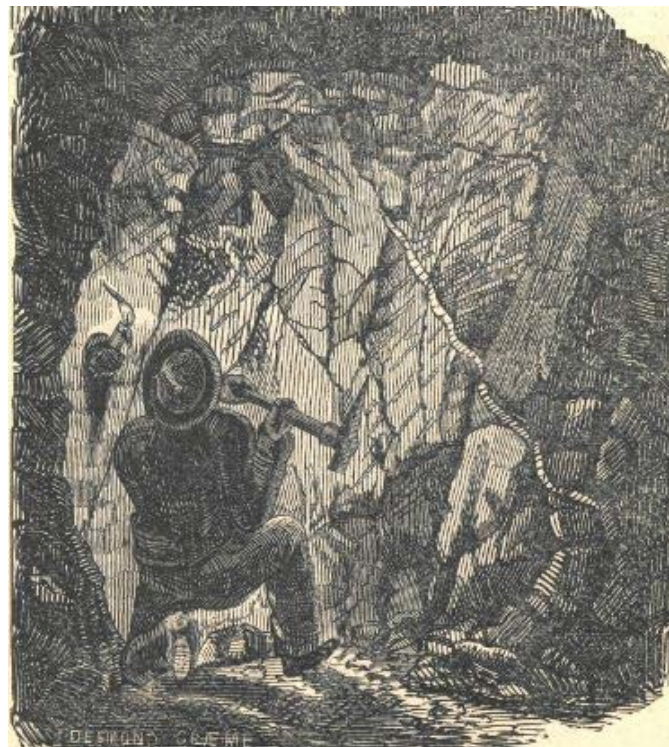
Mid 19 th century etching depicting miner working the ore vein in Ballygoneen mine, Glenmalure. Note the single candle providing the only source of light. Taken from 'The Mines of Wicklow' 1856. Author unknown.
