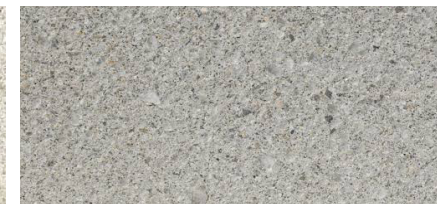
Shot blast concrete
