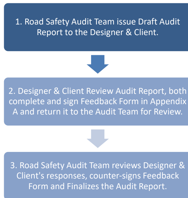
Figure 4.1 – Road Safety Audit Sign-Off and Completion Process
