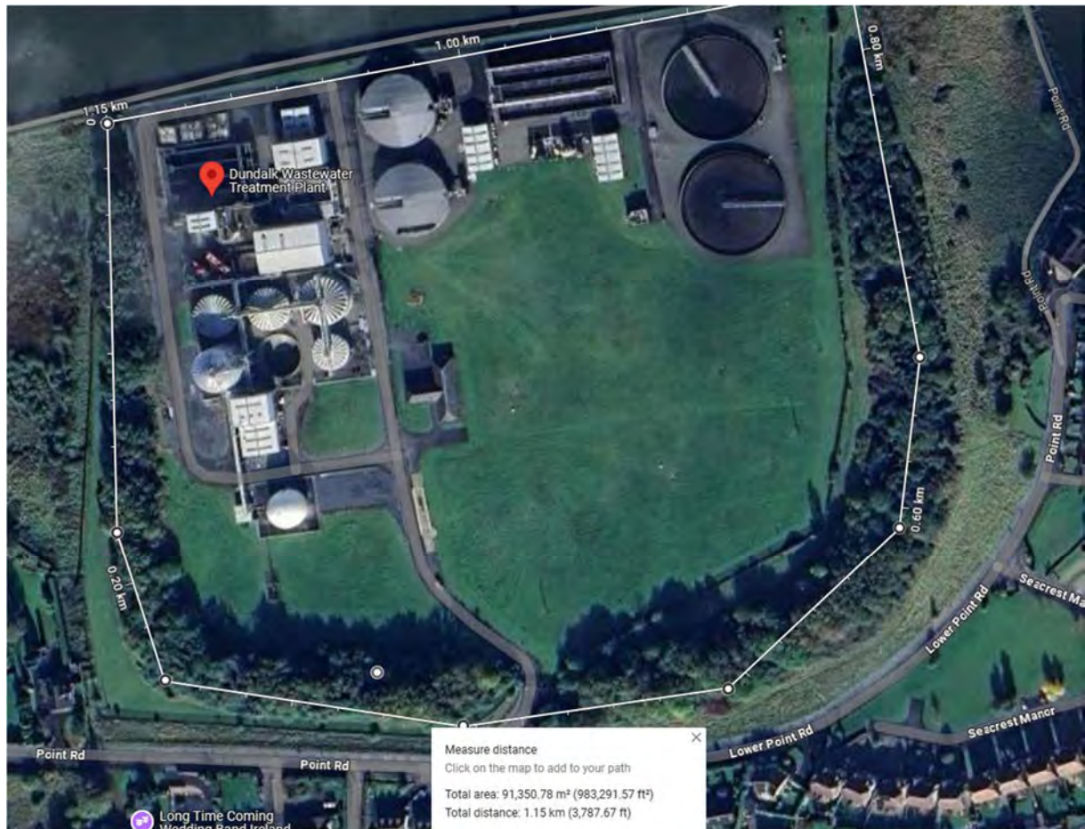
Image 13 Dundalk WWTP Existing WWTP Site Overall area coverage as measured 91,350m 2 Reported PE 220,000 Status Green \text{m}^2/\text{PE} = 91,350 / 220,000 = 0.41 \text{ m}^2/\text{PE}
